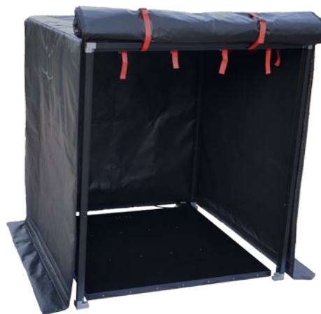
Camera calda Hot box
